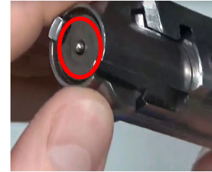
Step 12 : Show the firing pin
