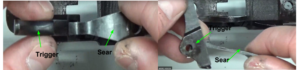
Step 23: Separate the trigger and the sear from each other
