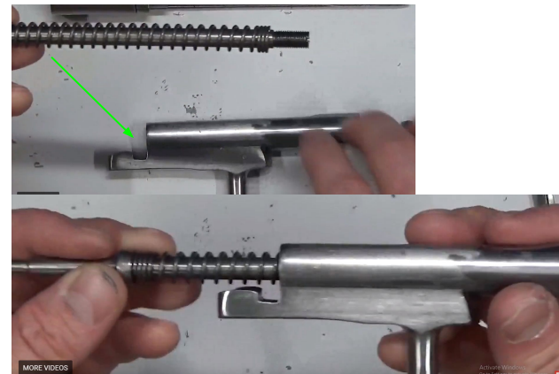
Step 47: Insert firing pin and spring into the bolt body
