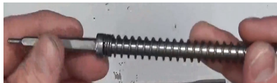
Step 47: Insert firing pin and spring into the bolt body
