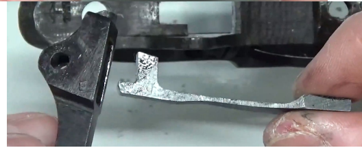
Step 24: Sand the back side on top of the sear on a 90 degree angle you can use your bench block. (Use small movements back and forth)
