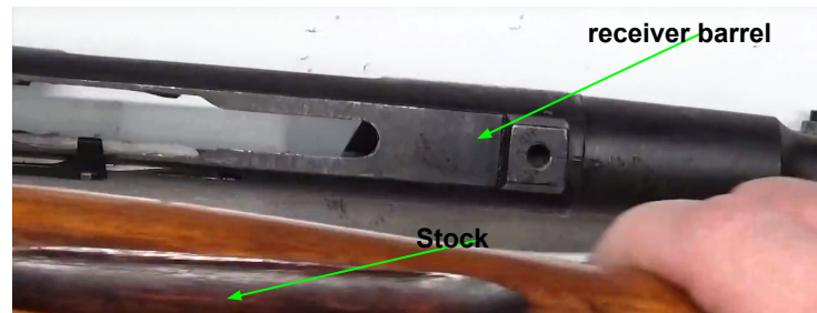
Step 9: Separate stock from receiver barrel, Place the firearm upright and let the weight from the receiver barrel separate from the stock
