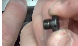
Step 24: Sand the back side on top of the sear on a 90 degree angle you can use your bench block. (Use small movements back and forth)
