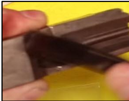
Step 74: Saturate the Bolt with CLP and Scrub it with your Brush.
