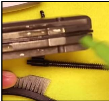
Step 74: Saturate the Bolt with CLP and Scrub it with your Brush.
