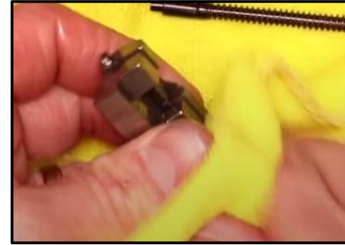
Step 76: Coat a Q-Tip in CLP. Use it to Scrub all the Tight Crevices of the Bolt.
