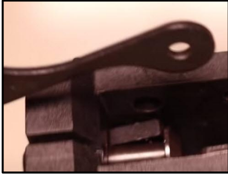
Step 54: Insert the Hammer Hinge Pin from the Back. Push down on the Straight Leg of the Spring and Let the Pin Overtop it to Capture it.
